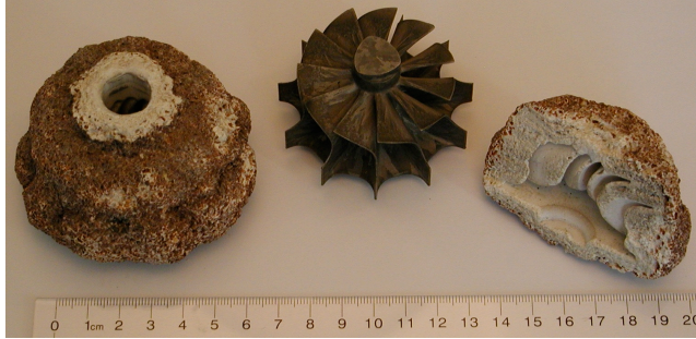
Fig. 1.4 Left to right: A ceramic mold after removal of the pattern; a superalloy turbocharger rotor (etched to reveal grain structure); and a half-section of a ceramic mold. Notice the smooth ceramic at the casting surface, giving way to a coarser consistency.
